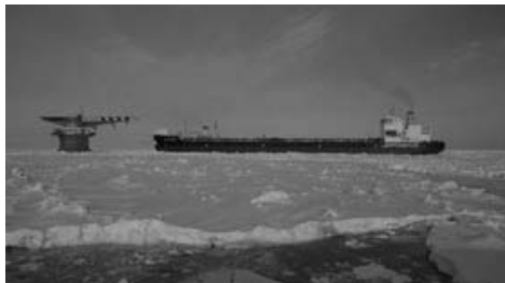
One of the ice-classed shuttle tankers operated by Sovcomflot loading oil at the Varandey offshore terminal.
