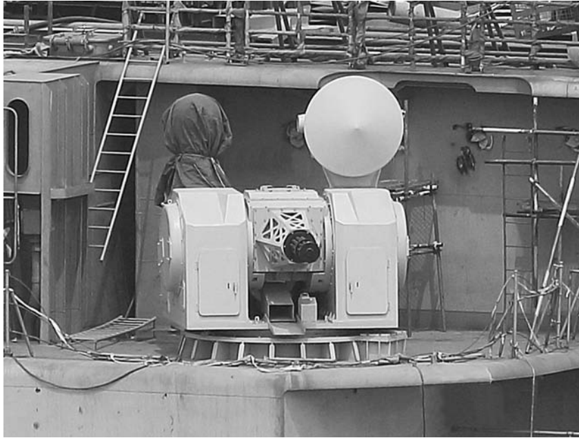
2011 Starboard Quarter images show a Type-1030 30mm CIWS & an FN-3000N missile system outfitted, the APAR & Sea Eagle Radar are also seen.
