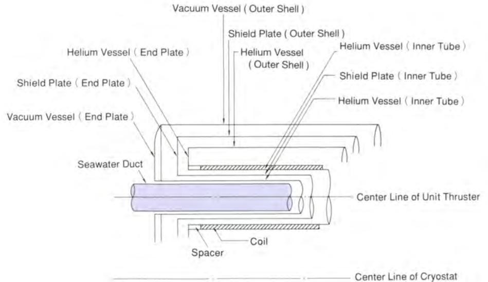
Fig. 5.3 Schematic illustration of the cryostat end structure
