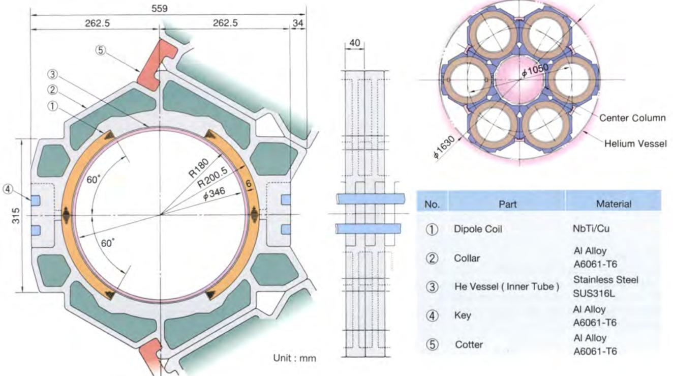
Fig.6.4 Coil holder (collar) details
