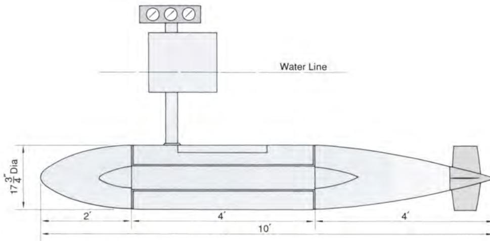
Fig. 1.1 Schematic drawing of the electromagnetic propulsion submarine "EMS-1" used by S. Way (1966)
