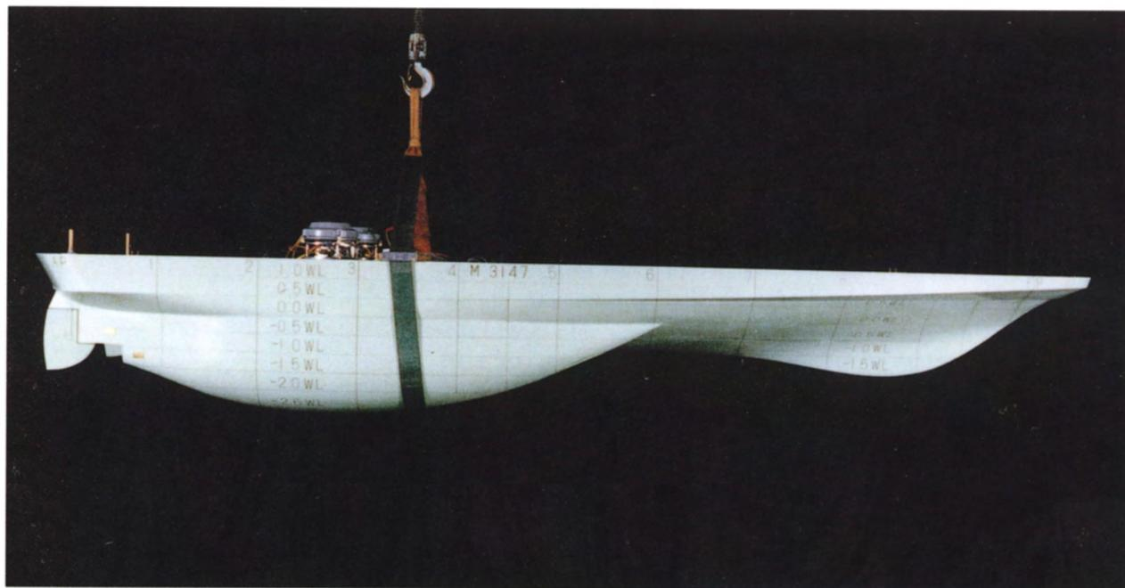
Photo 8.3 (a) The 1/8-scale model of the Yamato-1 used for tank tests
