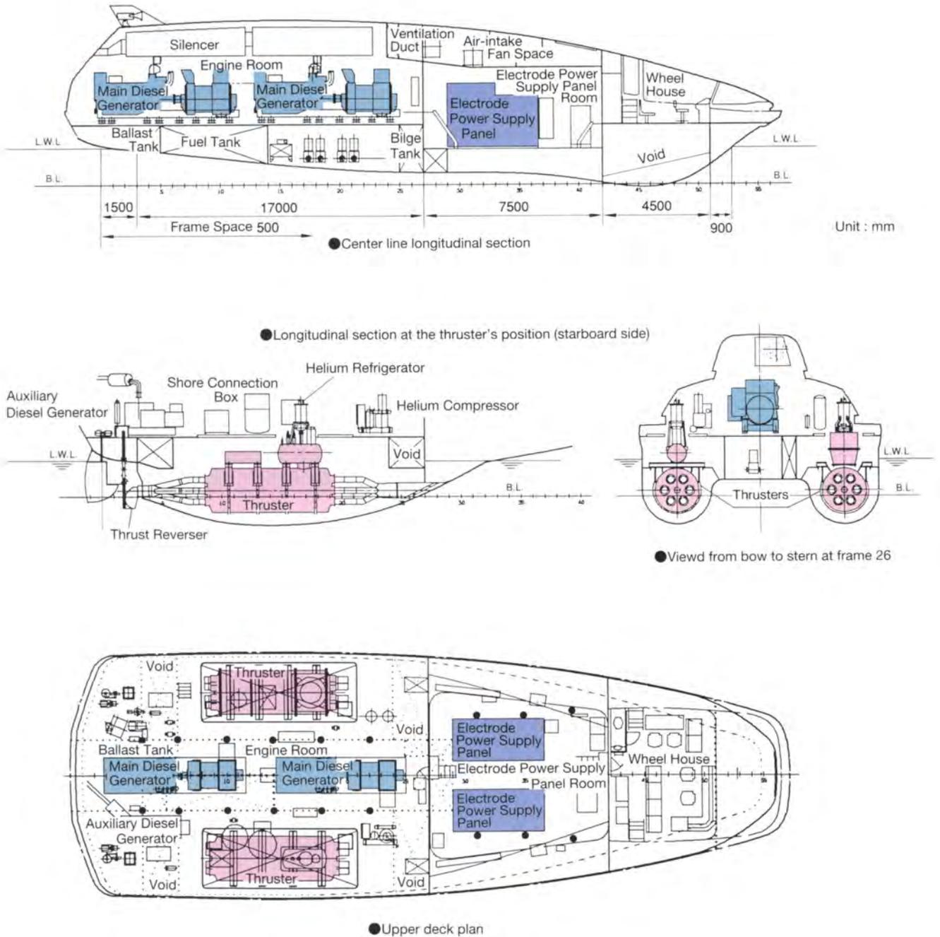
Fig. 2.1 General arrangement of the superconducting MHD propulsion ship Yamato-1
