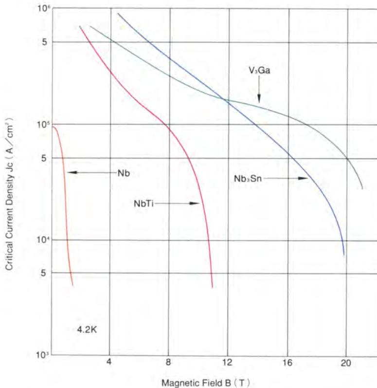
Fig. 4.3 Critical current density  $J_c$  vs. magnetic field magnitude  $B$  at  $T = 4.2$  K
