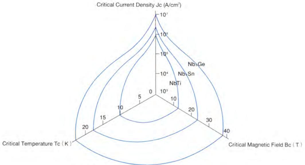
Fig. 4.2 Critical characteristics of superconductivity of easier-to-use Type II superconductors
