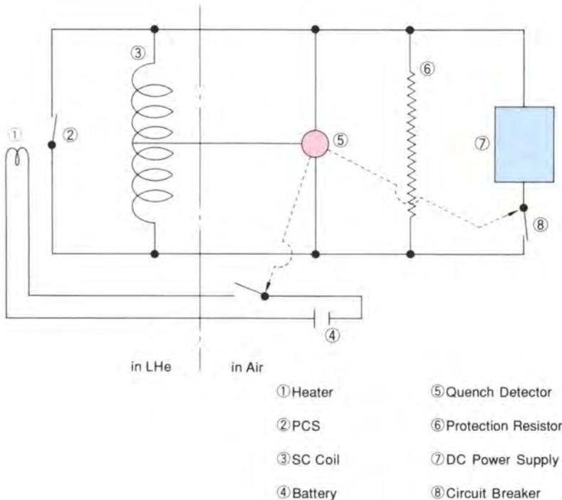
Fig. 10.5 Superconducting coil circuit
