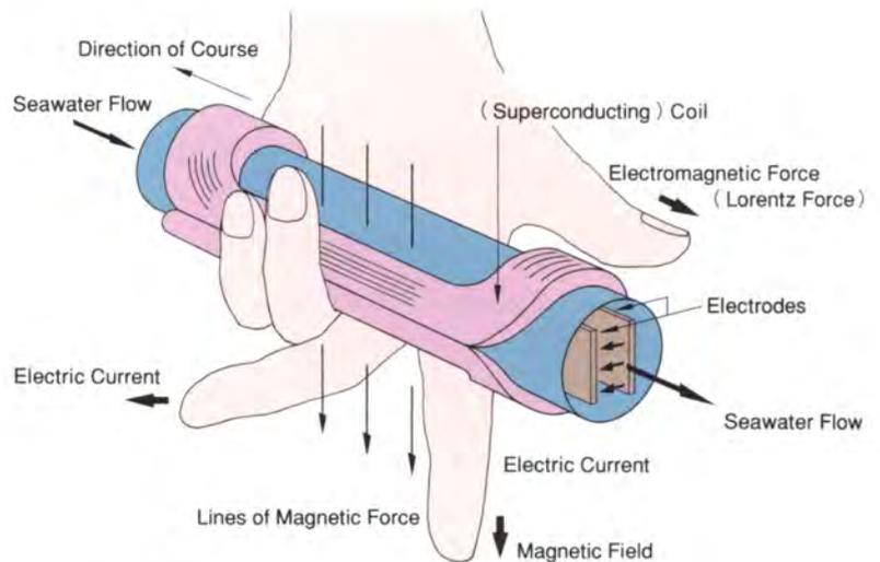
Fig. 3.2 The internal magnetic field-type MHD propulsion principle and Fleming's Left-Hand Rule
