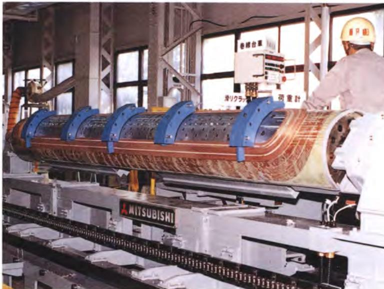
Photo 6.3 Coil winding operation using the winding machine
