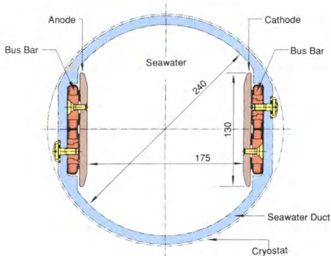
Fig. 7.2 Cross-section of a seawater duct
