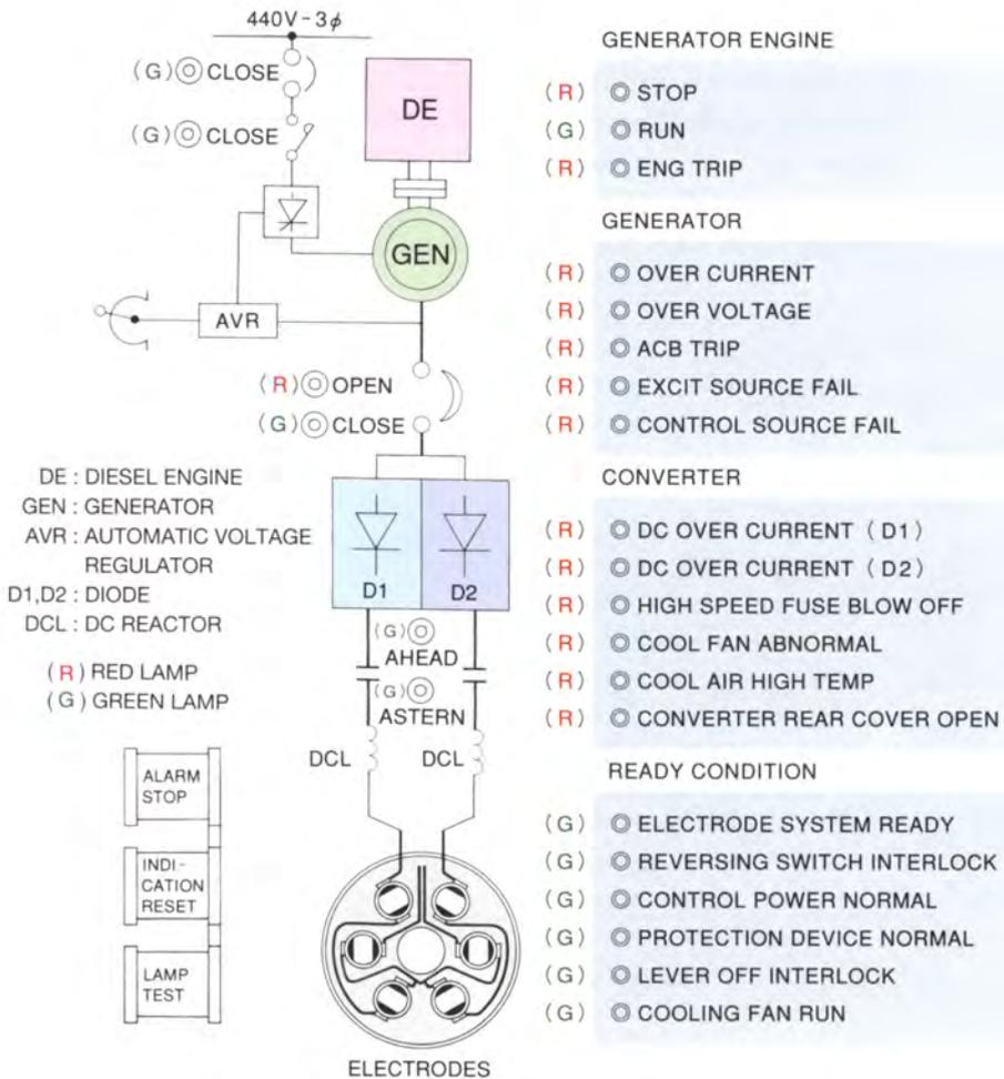
Fig. 7.5 Circuit diagram connecting the electrode power supply and the six sets of electrodes
