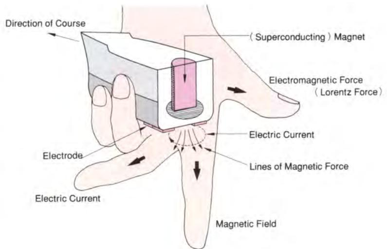
Fig. 3.1 The external magnetic field-type MHD propulsion principle and Fleming's Left-Hand Rule
