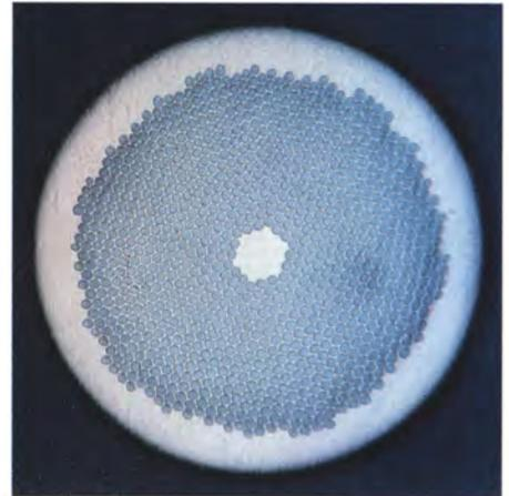
Photo 6.2 Cross section of a strand as a component of the superconducting cable; diameter of the actual strand is 0.85mm
