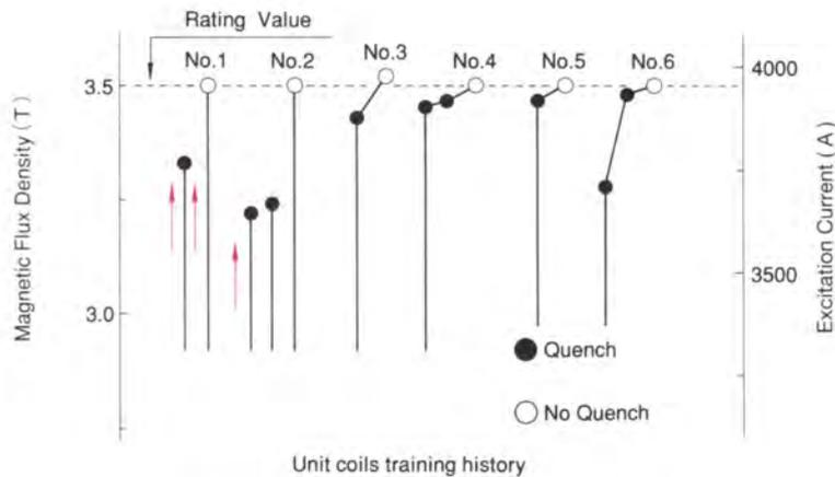
Fig. 8.2 Results of excitation tests on unit coils
