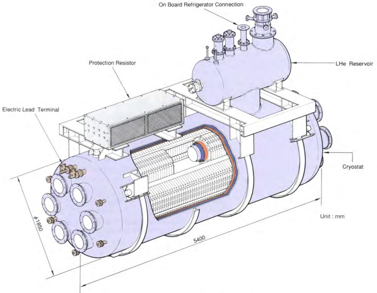
Fig. 5.1 Perspective cross-sectional drawing of the superconducting MHD thruster
