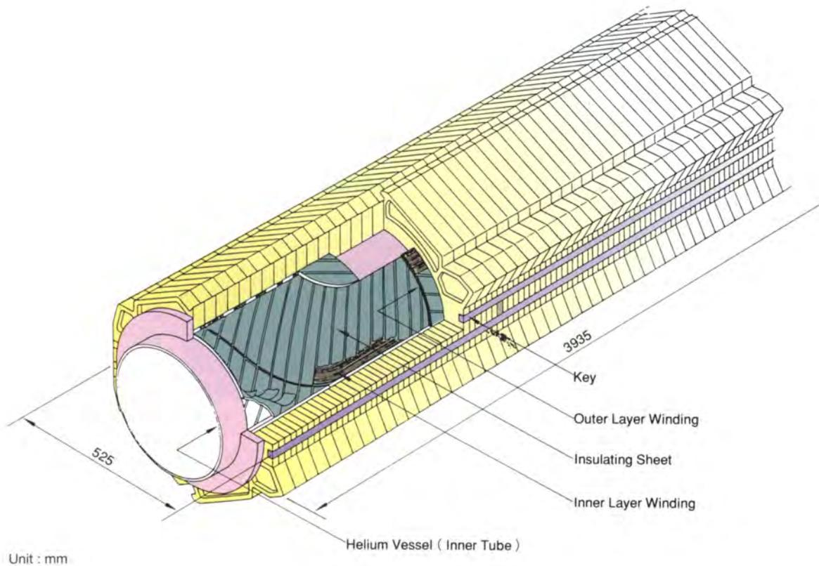
Fig. 5.4 Perspective cross-sectional drawing of a unit thruster
