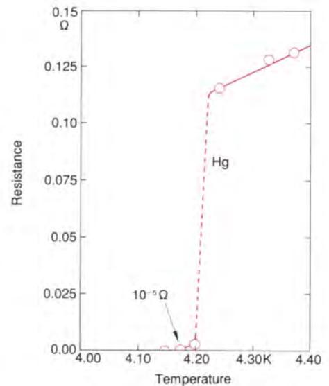
Fig. 4.1 Result of an experiment conducted by Kamerlingh-Onnes and his associates in 1911 on the relationship between electrical resistance and absolute temperature of mercury (Hg) (Recreated by referring to the figure included in "Superconductivity-Fundamentals and Applications" by Werner Buckel, VCH (1990))
