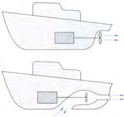
Figure : Screw propeller and water jet
