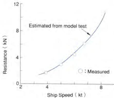
Fig. 10.4 Results of hull resistance measurements
