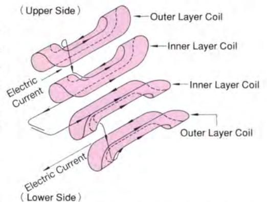
Fig. 6.2 Saddle-shaped coil pair construction
