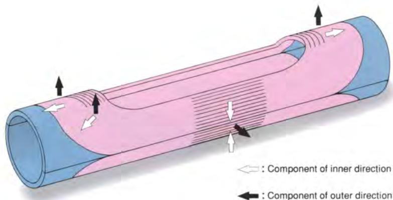
Fig. 6.3 Conceptual drawing of the electromagnetic forces acting on a saddle-shaped coil pair
