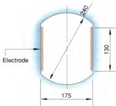
Fig. 2.4 Cross section of a seawater duct in the superconducting MHD thruster
