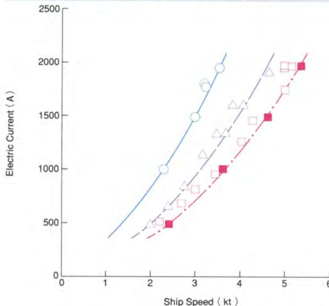
Fig. 10.2 Ship speed vs. electrode current at constant magnetic field intensity
