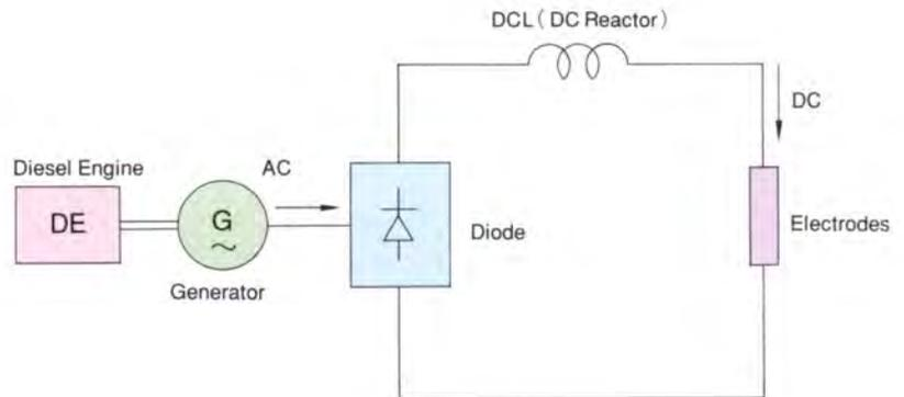
Fig. 7.3 Simplified circuit diagram of the electrode current supply
