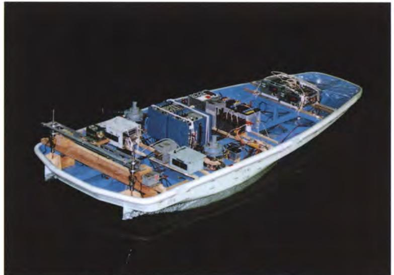
Photo 8.4 A maneuvering test using a model ship
