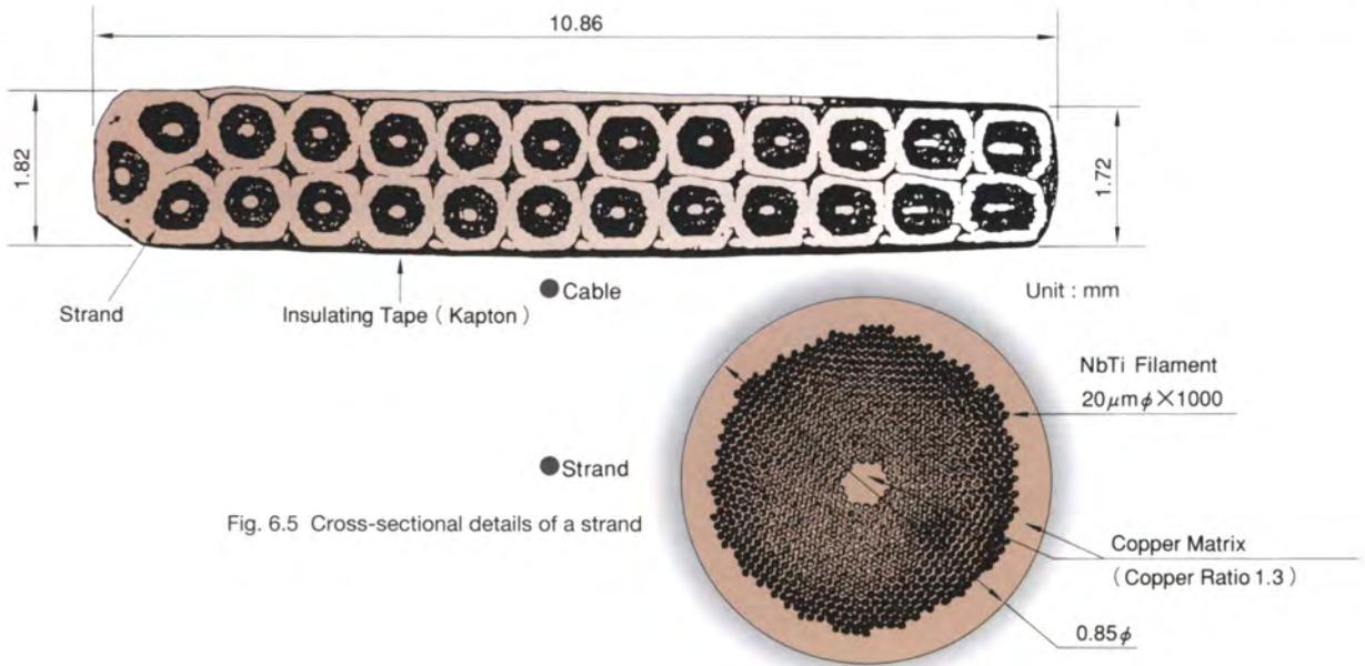
Fig. 6.5 Cross-sectional details of a strand
