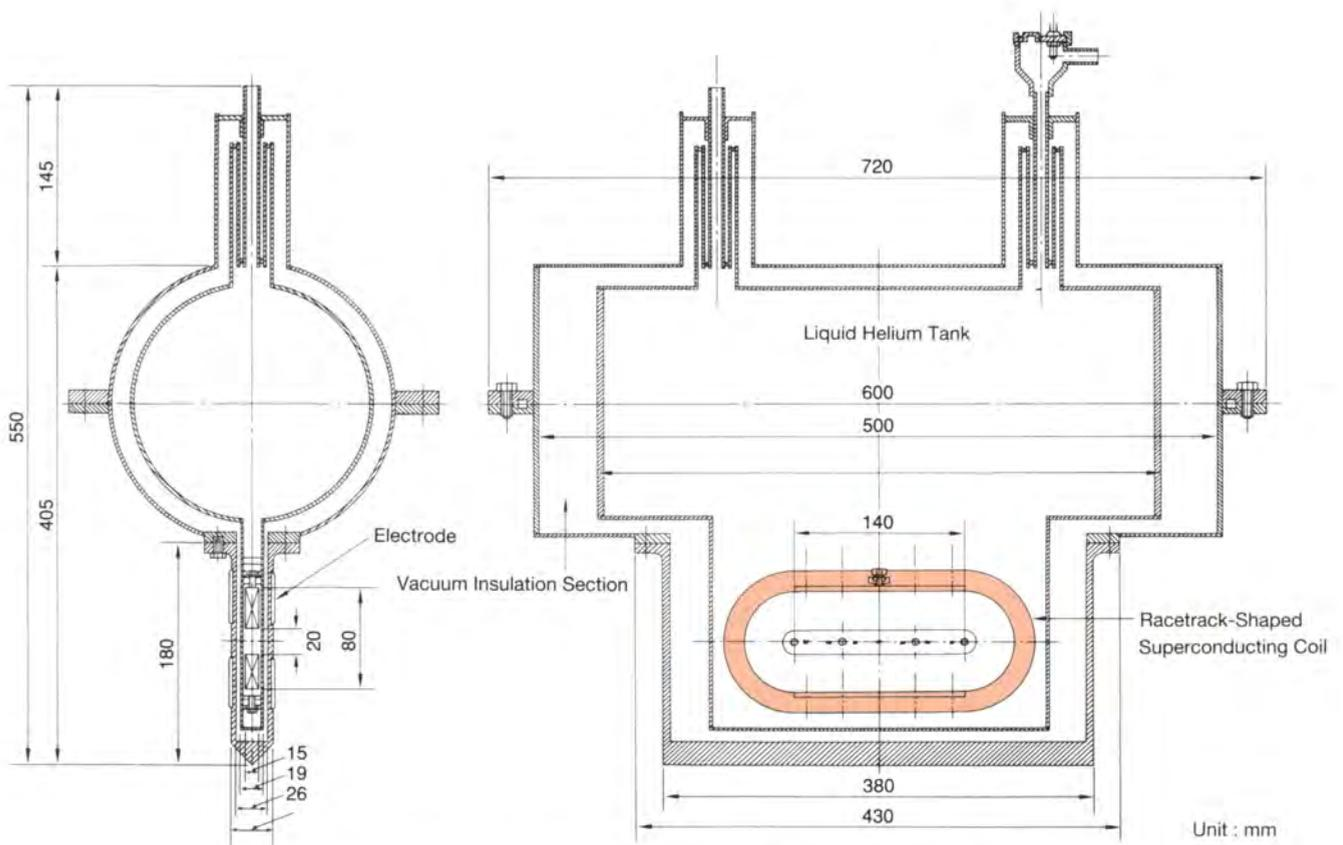
Fig. 3.3 Superconducting MHD thruster used for the model ship "SMED-1"
