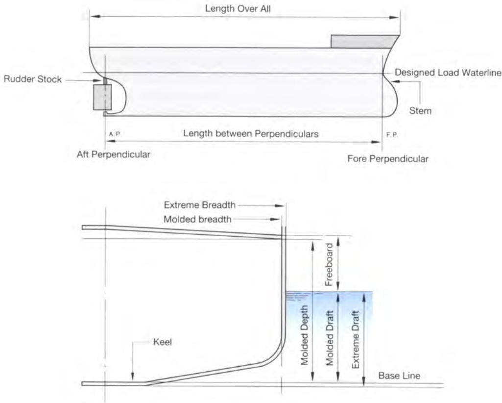
Fig. 8.1 Ship length, breadth, draft, etc.
