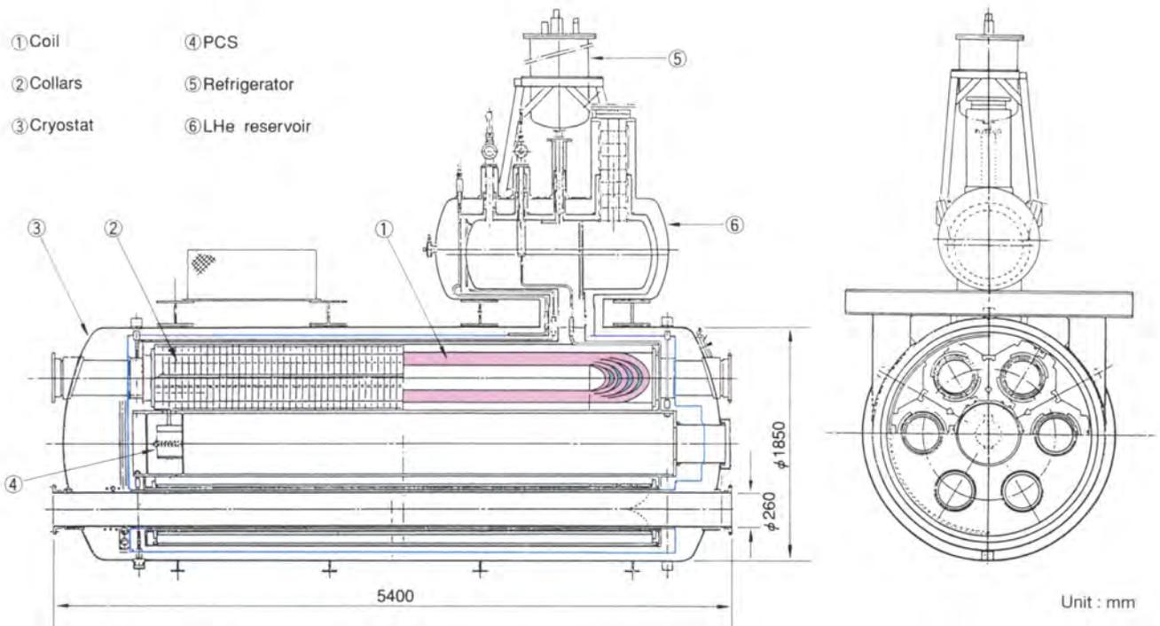
Fig. 6.6 Overall assembly of the superconducting MHD thruster before inserting the seawater ducts (made by Toshiba)
