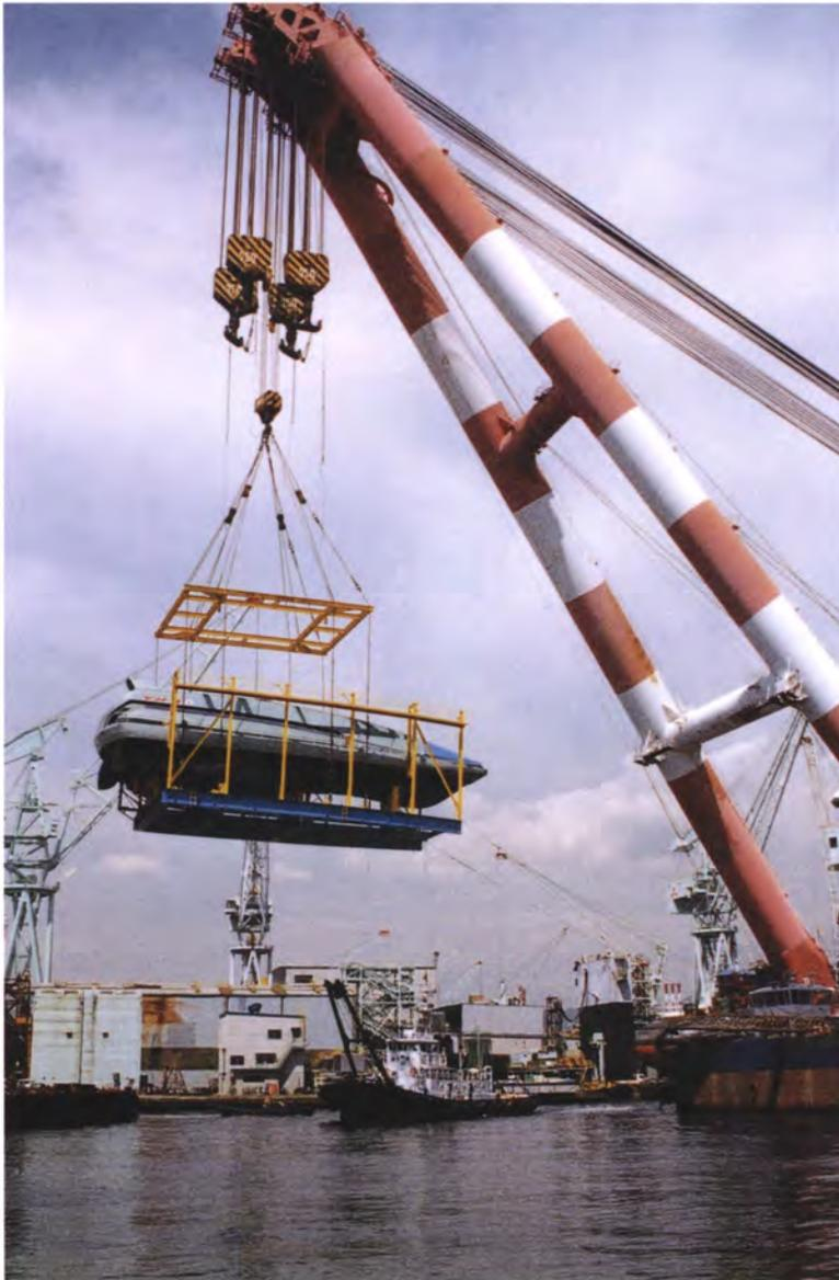
Photo 8.2 The Yamato-1 on the cradle is hoisted by a floating crane prior to launching her in the water
