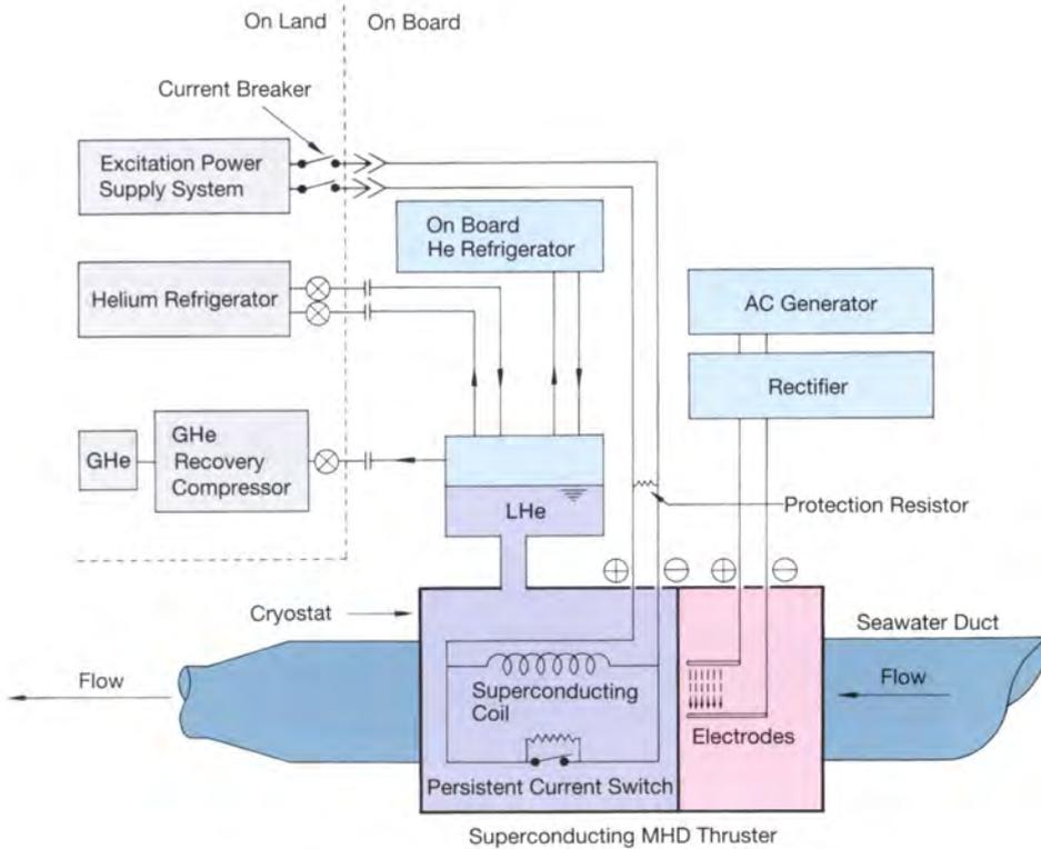
Fig. 9.1 Schematic diagram of the superconducting MHD propulsion system and land-based support facilities
