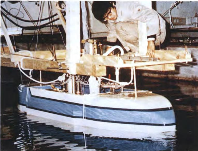
Photo 1.2 Superconducting MHD propulsion model ship "ST-500" running in the water tank at Kobe Mercantile Marine University
