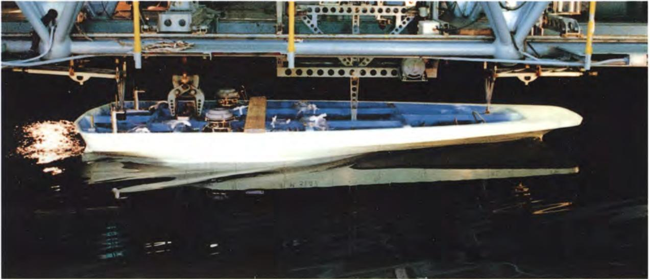
Photo 8.3 (b) A resistance test using a model ship
