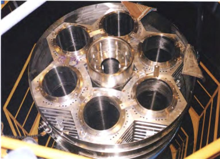
Photo 6.6 End section of the annular arrangement of the six coils. Each of the six coils is assembled into the annular arrangement by using the hexagonal collars inserted into the outer cylinder of the helium vessel. The end plate of the helium vessel is placed over this as a cap.
