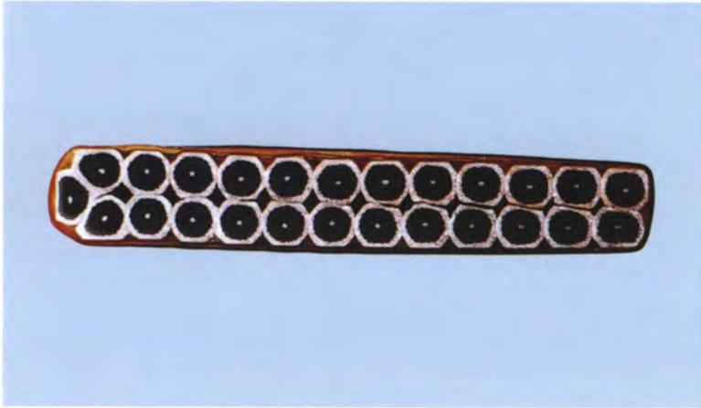
Photo 6.1 Cross section of the cable used as the superconducting coil (made by MHI)
