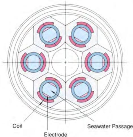
Fig. 2.3 Cross section of the superconducting MHD thruster
