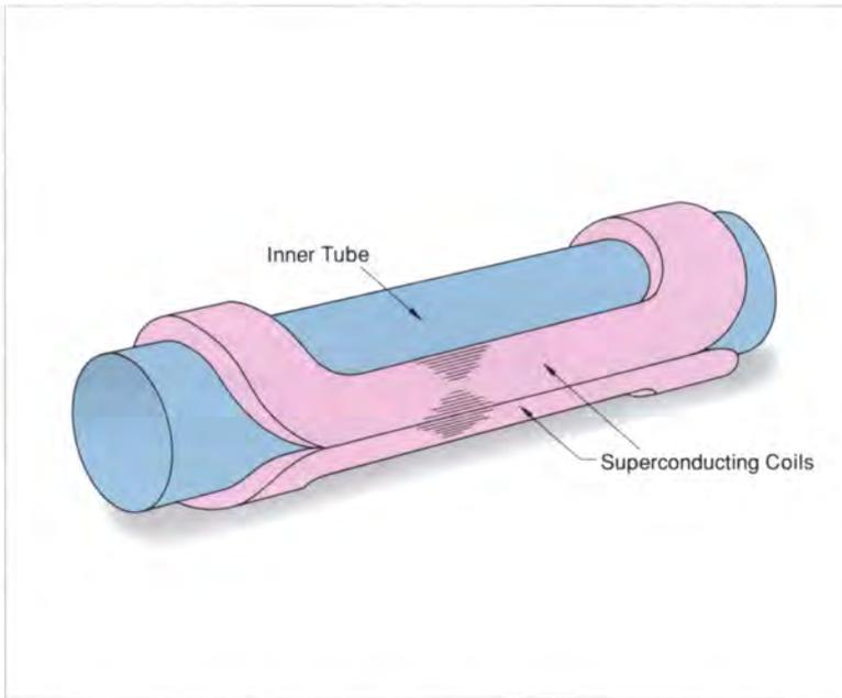
Fig. 6.1 Inner tube with a pair of saddle-shaped coils facing each other
