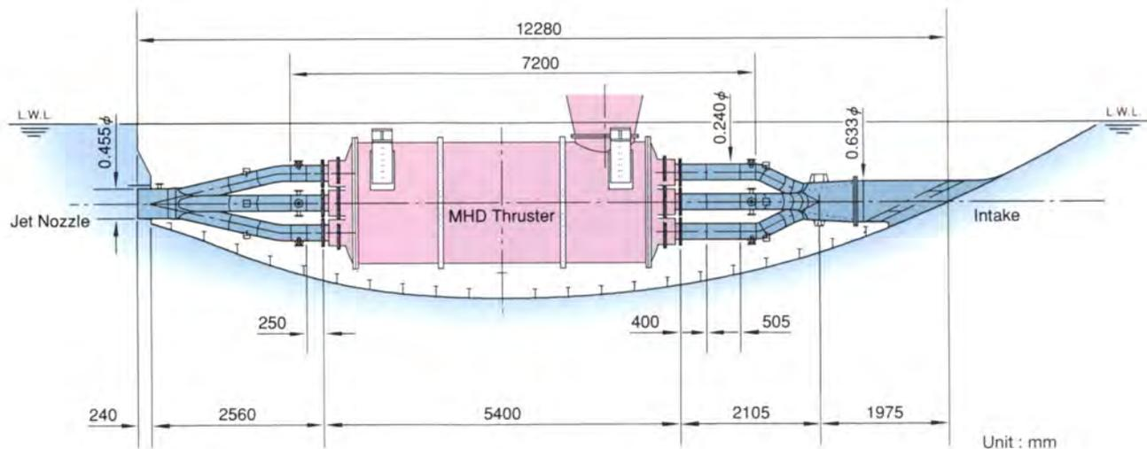
Fig. 2.2 Overall view of the superconducting MHD thruster and duct system housed in a bulge section
