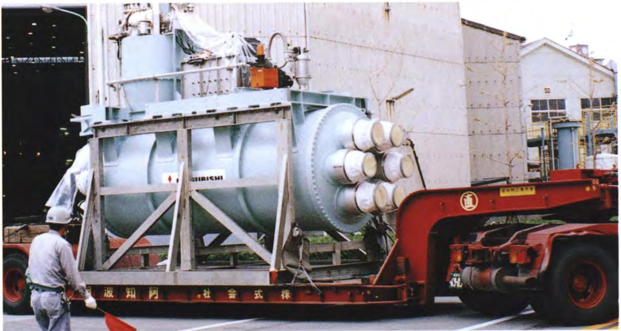
Photo 6.7 Overall view of the completed superconducting MHD thruster (made by MHI)
