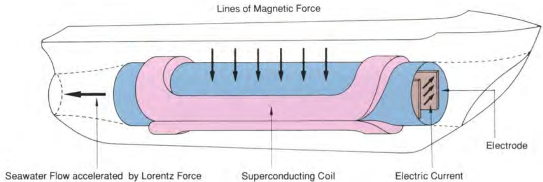
Fig. 3.4 Conceptual illustration of internal magnetic field-type MHD propulsion ship
