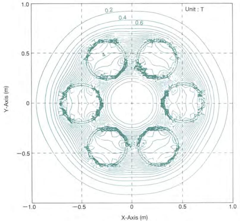
Fig. 5.2 Line drawing indicating the magnetic field magnitude distribution of the superconducting magnet in cross section
