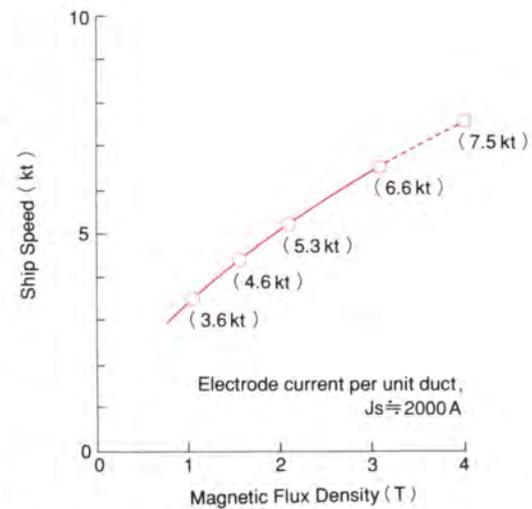
Fig. 10.3 Ship speed vs. magnetic field magnitude at 2,000 ampere electrode current
