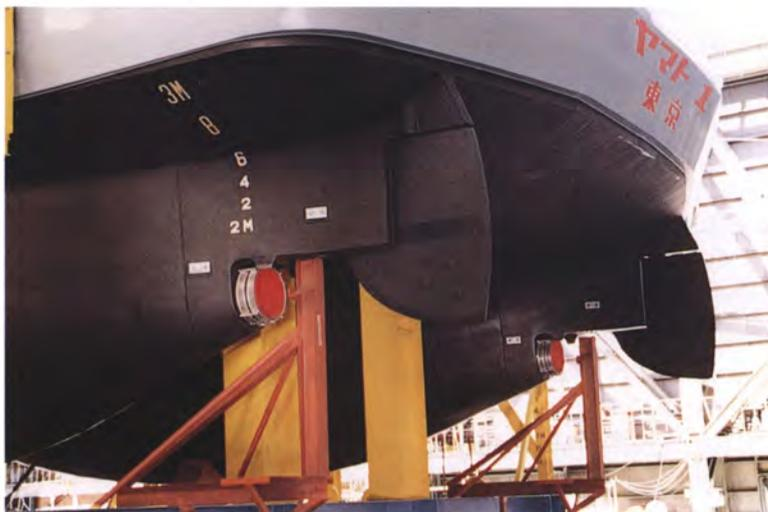
Photo 2.3 Seawater intake and nozzle of the Yamato-1
