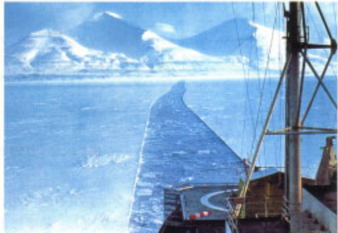
Figure 4.1-14 Channel formed by a WAAS ship
