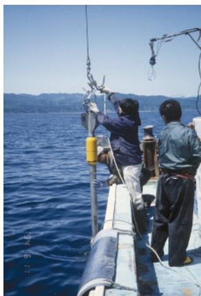
Sediment sampling by gravity corers
