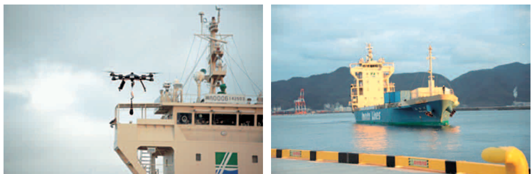
Figure 2-4 An unmanned drone carrying a heaving line upon docking of the Mikage and the Sunflower Shiretoko autonomously docking at Oarai
