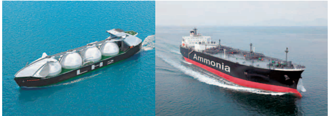
Figur 1-2-2 Large liquified hydrogen carrier (left) and ammonia powered ammonia carrier (right) Photos courtesy of Kawasaki Heavy Industries (left) and NYK Line (right)
