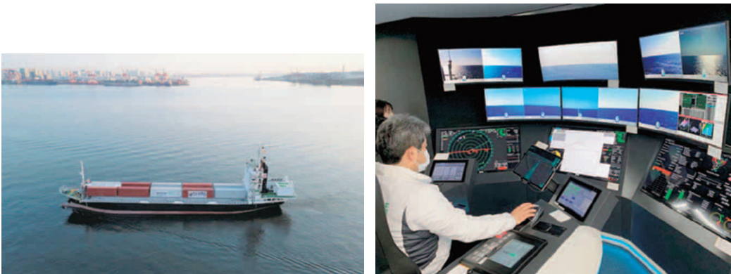
Figure 2-5 Suzaku, operating in Tokyo Bay and the land-based remote operation support center
