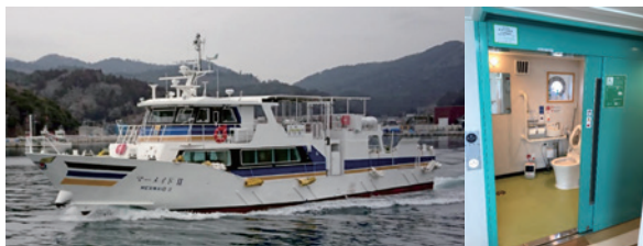
The hull of "Mermaid II," (Ajishima Line Co., Ltd.) a vessel subsidized in fiscal year 2018. The photo on the right shows the ship's barrier-free lavatory (the entrance and exit doors are automatic for easy access by wheelchair users, and the lavatory has space for wheelchairs to turn).
