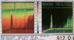
A methane plume from the sea floor, visualized using the fishery echo sounding method. It rises some 600m from the sea floor at a depth of 912.0m, reaching a depth of around 300m.
