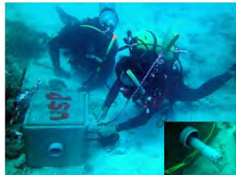
Beqa SBE-56 Logger Deployment
