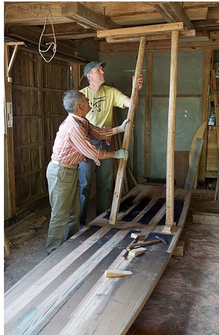
left : An adze with a uniquely curved handle is used. right : Mr. Murakami and the author doing the "kikoroshi," or propping the bottom plank in place. (Photo by Angela Robins).
