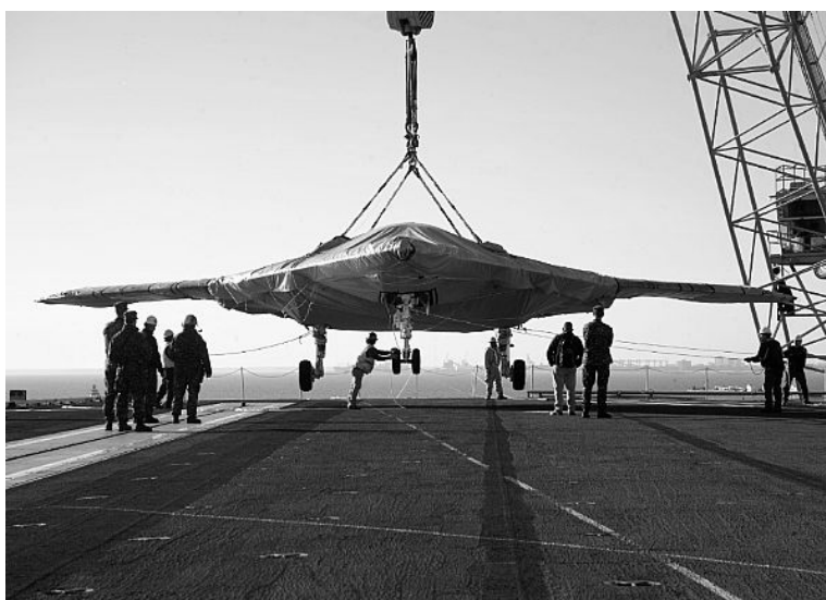
U.S. Navy Sailors assist with the onload of the X-47B Unmanned Combat Air System (UCAS) demonstrator aboard the aircraft carrier USS Harry S. Truman (CVN 75)
