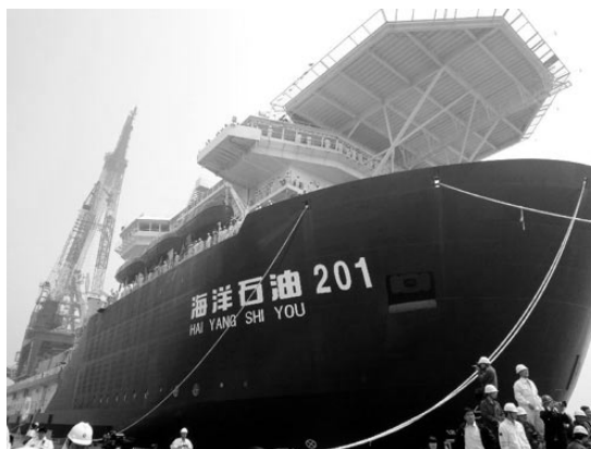
The newly-built deepwater pipelay crane vessel "Hai Yang Shi You 201"
