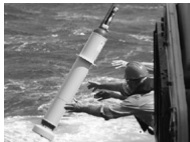
Deploying an Argo ocean profiler
