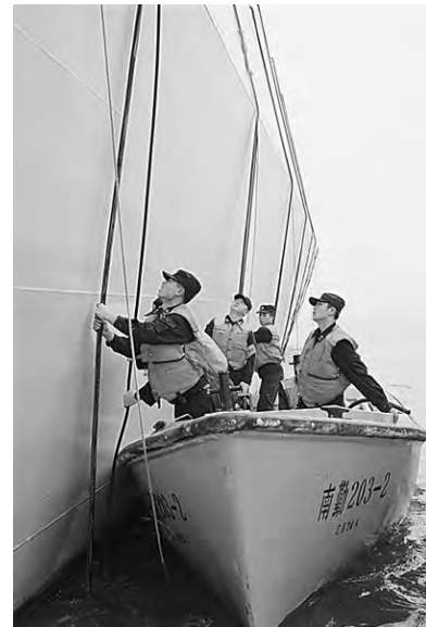
Adjusting demagnetization cables
