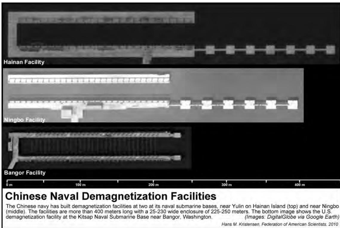
China's two known naval demagnetization facilities are similar, capable of handling all Chinese submarine sizes, and similar in design to U.S. demagnetization facilities.
