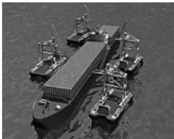
A computer simulation demonstrates how smaller ships could unload containers from a larger cargo ship at sea
