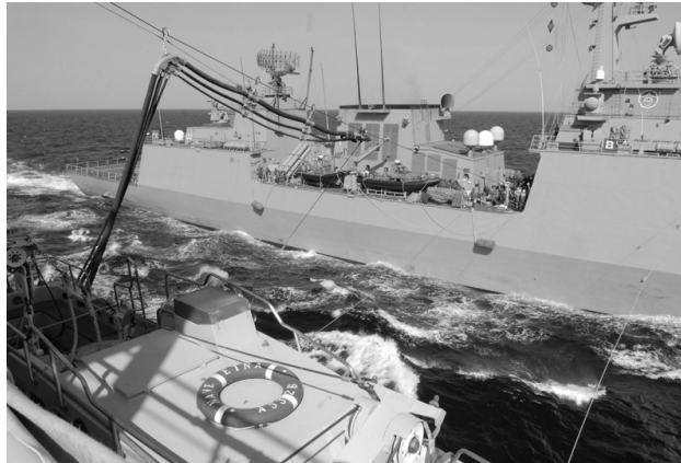
Italian ship Etna (Front) refueling Korean warship Yi Sunshin (back) at Sea
