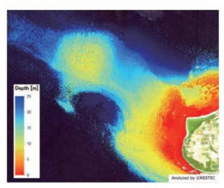
Figure 1-14 Coastal bathymetry derived from satellite Images
