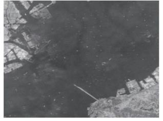
Figure 1–12 Radar image of vessels in Tokyo Bay taken from ALOS2 (*Daichi* 2)
