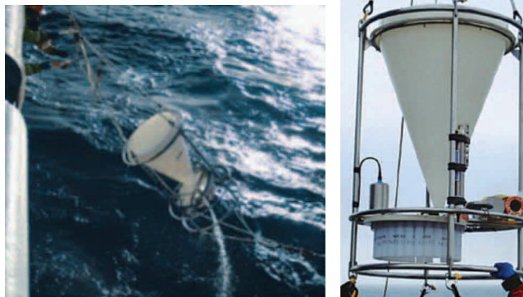
Figure 1-8 Sediment Trap Mooring System to sample falling solid particles in the ocean.
