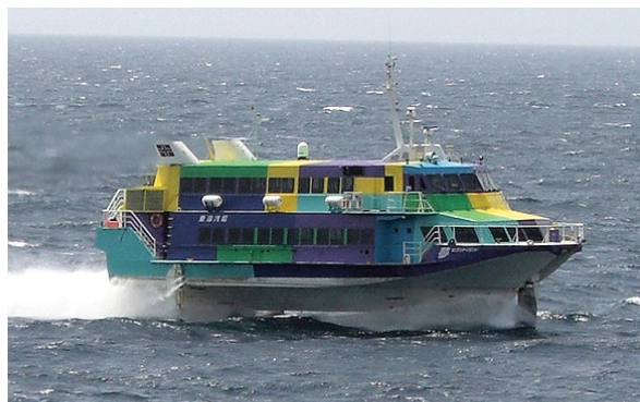
■Figure 1. Hydrofoil type high-speed vessel. Employed on important high speed routes linking remote islands with the mainland.
