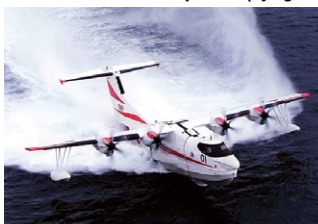
Cruising range: at least 4,500km, maximum take-off and landing weight (land): 47.7 tons, maximum take-off and landing weight (water): 43.0 tons, maximum take-off distance: 280m, maximum landing distance: 310m, maximum wave height: approx. 3m. (Photo courtesy: ShinMaywa Industries, Ltd.)
