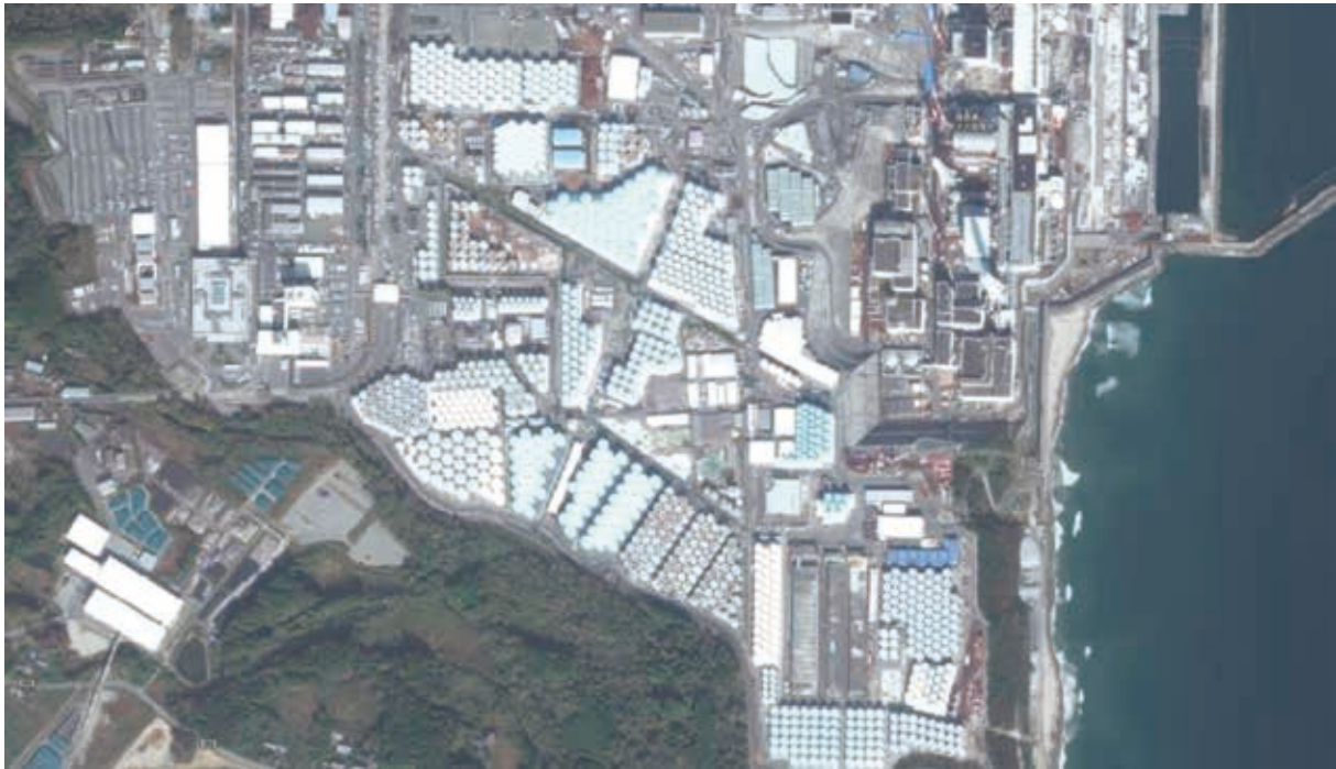
Photo 1: Fukushima Daiichi NPS filled with ever-increasing number of tanks holding ALPS-treated water
