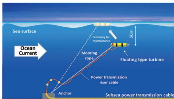
operated at a stable depth without being affected by waves, and they will not interfere with ship navigation. Furthermore, since it is possible to use simple mooring, the ease of installation also contributes to cost reduction.
