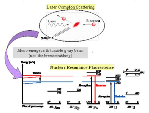
Figure 5-1. Gamma ray creation and nuclear resonance fluorescence using Laser-Compton scattering
