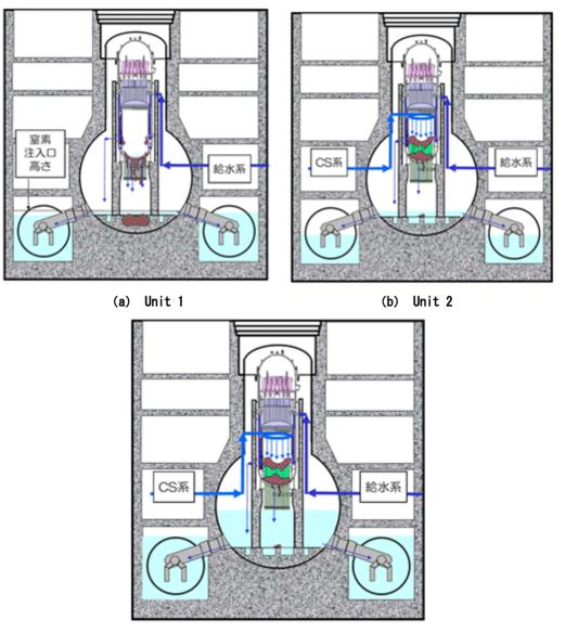
Figure 1-3. Estimation of conditions in reactor cores
