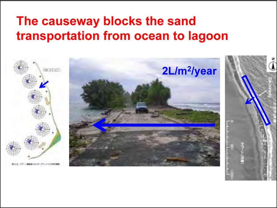
Figure 7. Foraminifera are densely populated on the outer reef flat with a production rate of 2L/m^2/year . However, the causeway blocks the sand transportation from ocean to lagoon.
