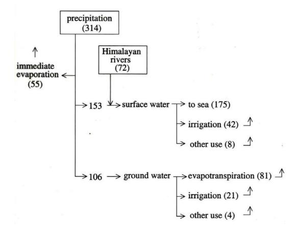
Figure 4: India's annual water budget. The unit is 10<sup>10</sup> m<sup>3</sup>. The area covered for this budget is south of Himalayan foot-hills and is approximately 3 x 10<sup>6</sup> sq. km. Monthly-mean precipitation data are from Indian Institute of Tropical Meteorology, Pune (Parthasarathy data set). Evaporation data are from NCEP/NCAR reanalysis (Kalnay et al., 1996) Other data were taken from: Agarwal and Narayanan (1999), Nag and Kathpalia (1975), and Rao (1979)
